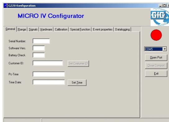
The MICRO IV is put in such a way now into the Slot of the data interface that the diffusion opening lies over the two gas connectors in the data interface. For connection the middle key must be pressed at the MICRO IV. The circle becomes green to indicate that the connection is completed. On the present page in the program the fields are filled with the data by the MICRO IV.
